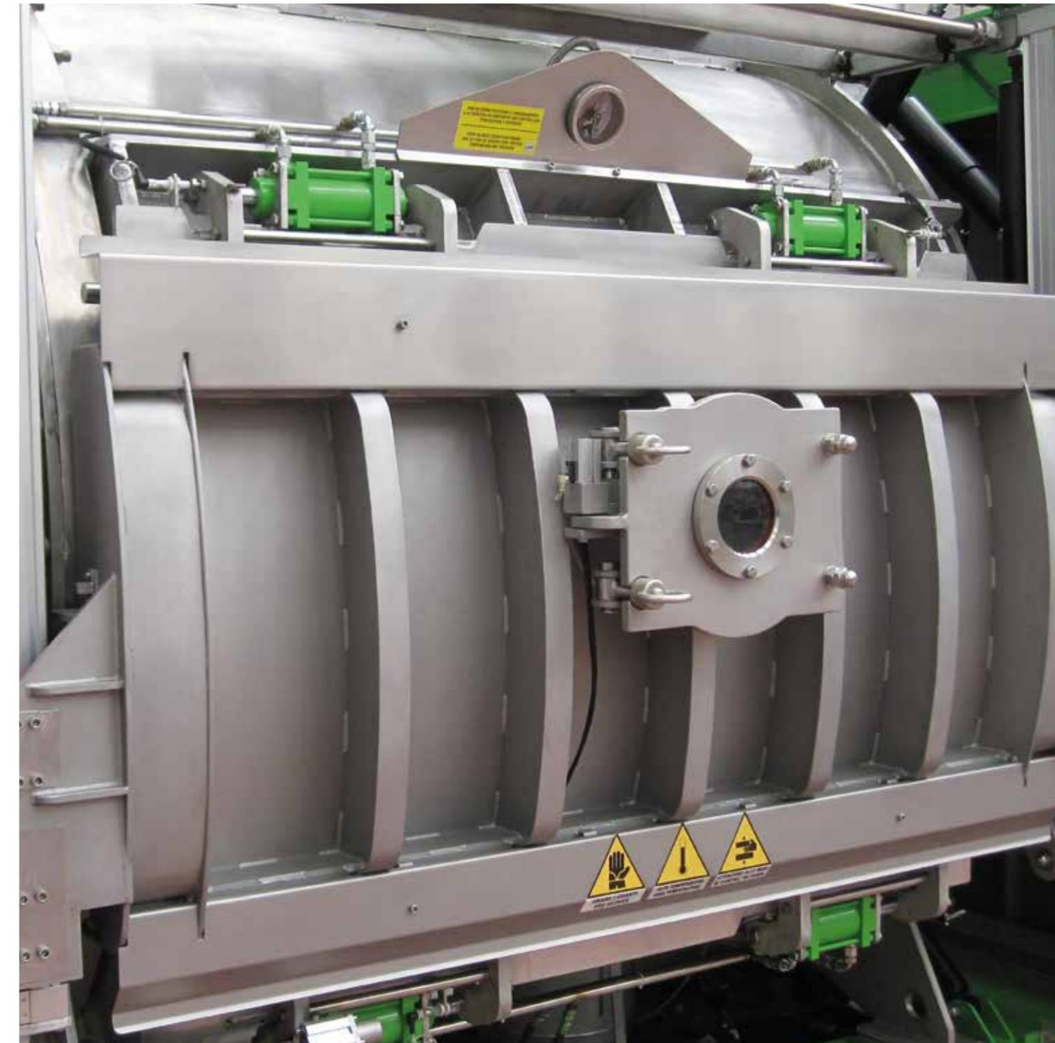
MACCHINA ROTATIVA PER LA TINTURA DI CAPI CONFEZIONATI, CALZE E SEAMLESS CON SISTEMA DI CARICO E SCARICO FACILITATO.
